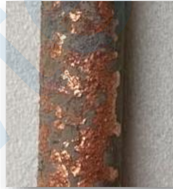
General copper tube and the corrosion-resistant tube we use after corrosion test
