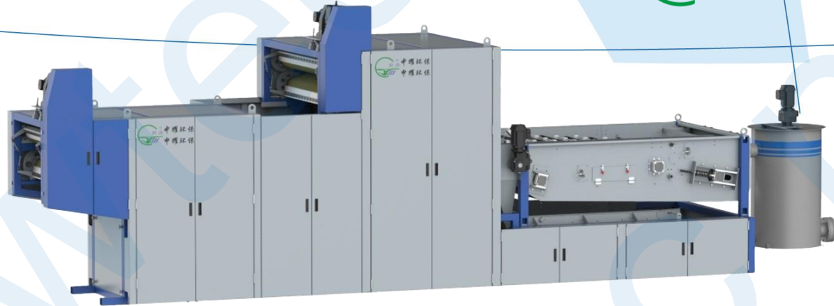
Thickening + Primary Belt Filter Press + Secondary High Pressure Belt Filter Press
